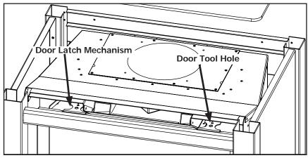
Figure 17. Top latches for glass door
