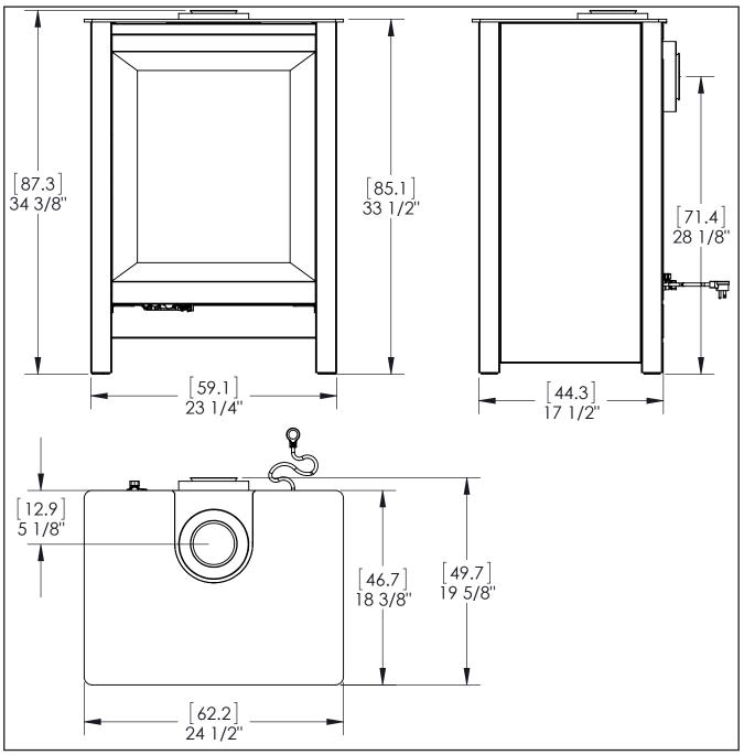
Figure 1. S20I/ S20ID Dimensions - Top Vent
