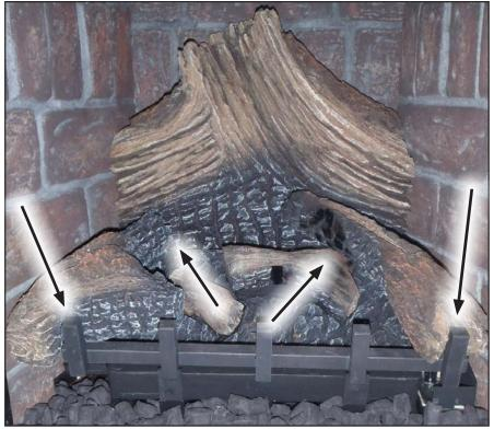
**Step 3**: Install the big y shaped twig on the far left side by locating the bottom of it on the far left log grate upright. The twig should run parallel with the side of the firebox and the top will rest on the top of the ember bed. Then install the big, slightly curved twig on the far right side by locating the bottom of it on the far right log grate upright. The top will rest on the smooth section of the middle ember bed twig.
