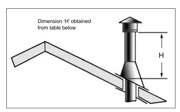
Figure 36: Height of Vertical Termination; Reference Table 7.
