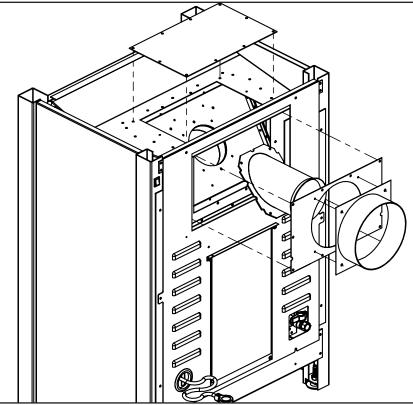
Figure 25. Vent Conversion - Step 3
