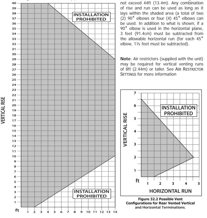
HORIZONTAL RUN Figure 32.1 Possible Vent Configurations for Top Vented Vertical and Horizontal Terminations.
