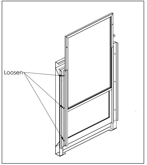
Figure 48. Safety Screen Removal
