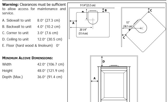
Figure 22 Clearance to Combustibles
