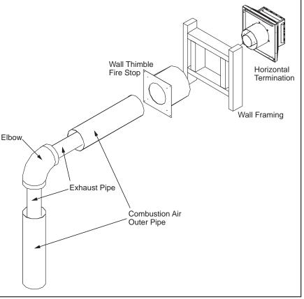
Figure 34. Horizontal Vent Termination
