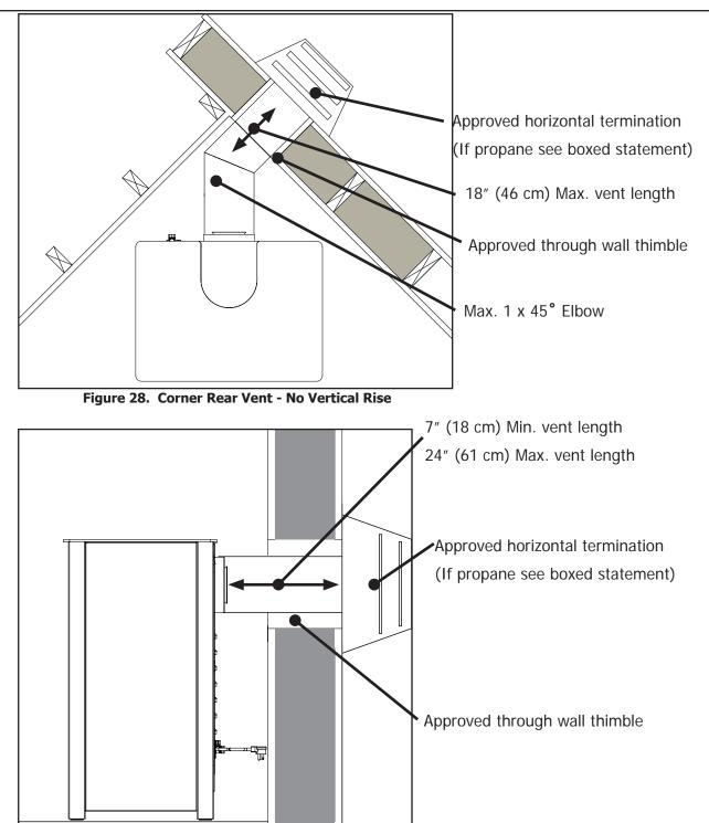
Figure 29. Flat to Wall Rear Vent - No Vertical Rise
