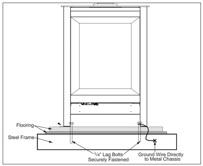
Figure 30: Correct Mobile Home Installation
