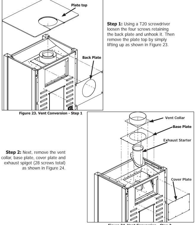
Figure 24. Vent Conversion - Step 2
