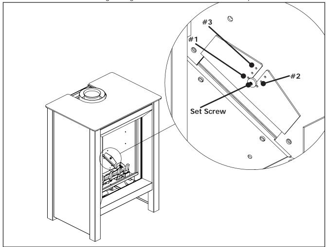
Figure 33: Installation of Air Restrictors
