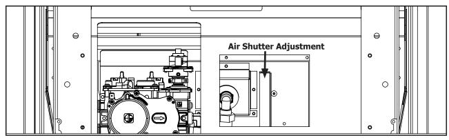
Figure 3. Air shutter adjustment lever.
