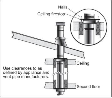
Figure 38: Multi-Story Vent Pipe Installation.
