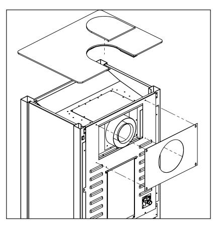
**Step 4:** Re-install the plate top by aligning the bolt heads on the bottom side with the rear mounts (see Figure 23). Re-install the back plate and tighten the four retaining screws. Finally, install the plate vent cover supplied with the S20I/ S20ID as shown in Figure 26.
