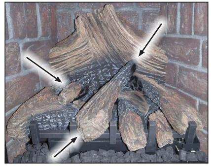
**Step 5**: Finally, install the large straight twig between the center and left side log grate upright by locating the notch on the bottom side with the log grate cross bar. The top of the twig will rest on top of the far right curved twig. The last remaining straight twig gets intalled by locating the front in the crook of the far left y shaped twig and the back notch rests on the top edge of the ember bed.
