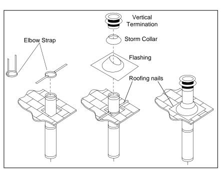
Figure 35. Vertical Vent Termination
