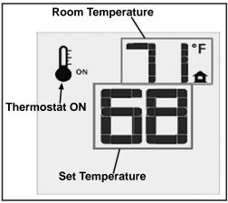
Figure 9: Remote Control Displays Set Temperature.
