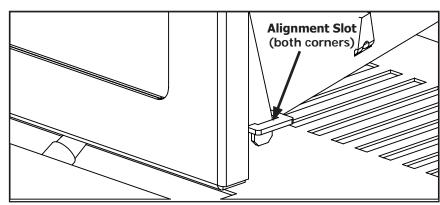
Figure 18. Bottom Alignment Slots for glass door
